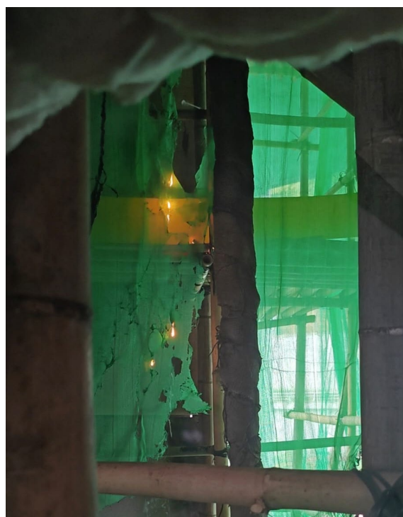
Photo 2-11 (b): Fire Spread in Test 7 Using Non-FR Safety Nets
