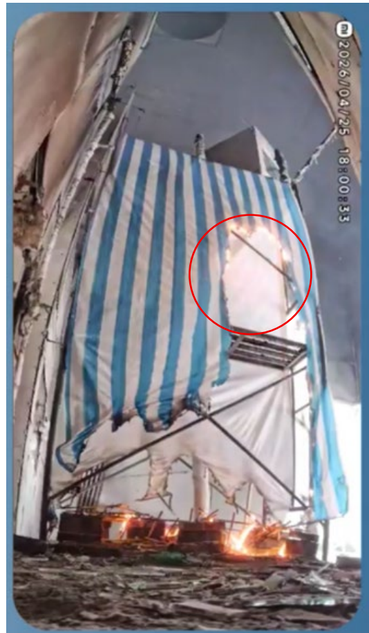
Photo 2-10 (ad): Extensive Fire Spread on Non-FR Canvas (White & Blue Striped)
