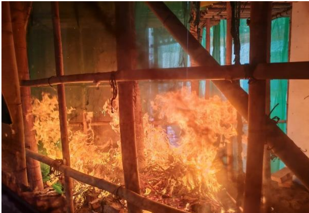
Photo 8-2 (c): Fire Developed from a Small Fire Source During Fire Tests
