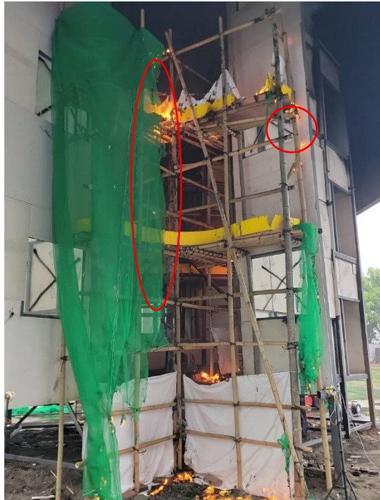
Photo 7-6 (c): Fire Spread Along Safety Nets in Test 12
