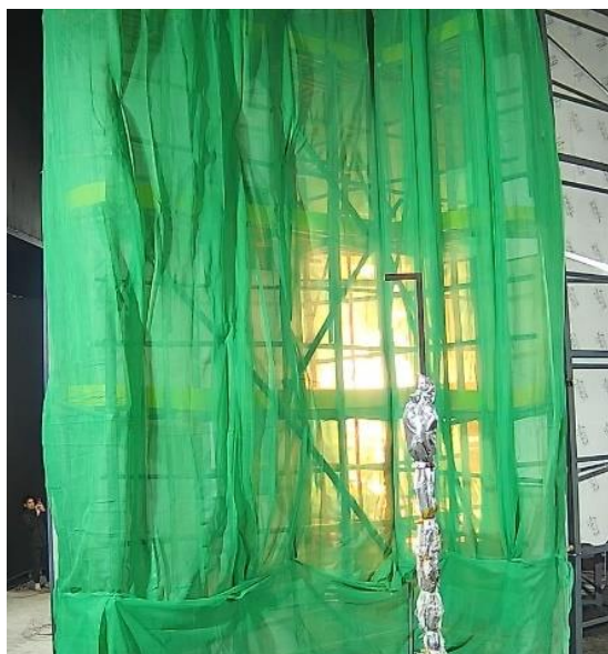
Photo 7-3 (a): The Fire Condition at 30 Mins With HRR at About 1MW
