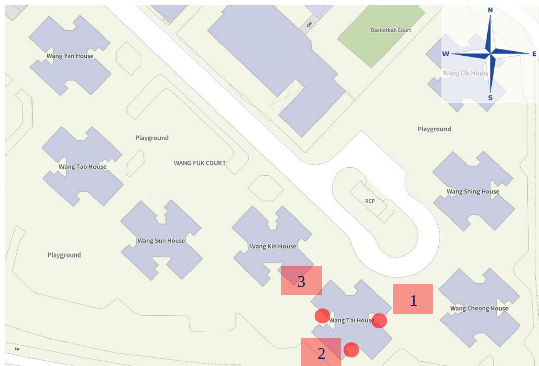
Figure 5-13: Map Indicating the Fire Spread Along Re-Entrants at Wang Tai House
