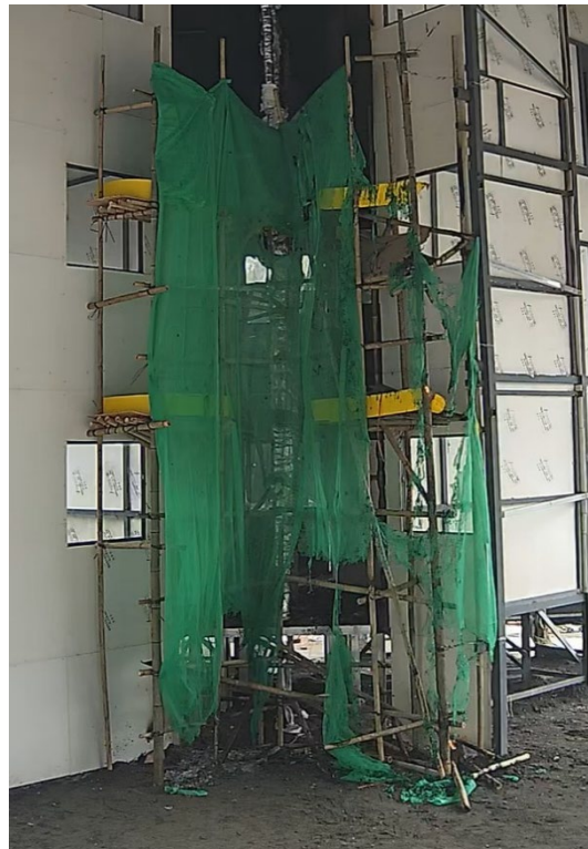
Photo 2-16 (d): Post-Fire Condition in Test 3 [Sample 1 (Uncertified)]
