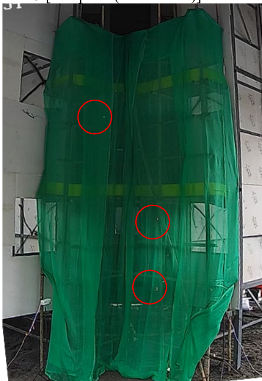
Photo 2-16 (g): Secondary Ignition in Test 7 [Sample 3 (Non-FR)]
