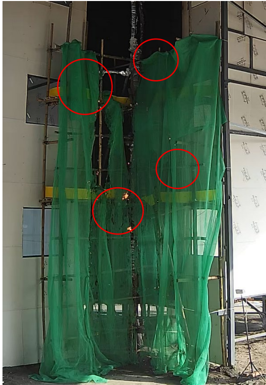
Photo 2-16 (a): Secondary Ignition in Test 1 [Sample 1 (Uncertified)]
