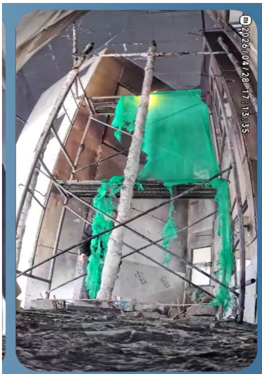
Photo 2-10 (aa): Post-Fire Condition of Sample 3 (Non-FR) (53 min)
