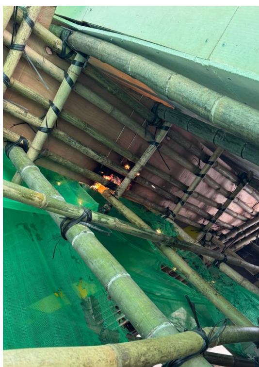
Photo 2-1 (a): Fire Spread to Wooden Plank in Test 1
