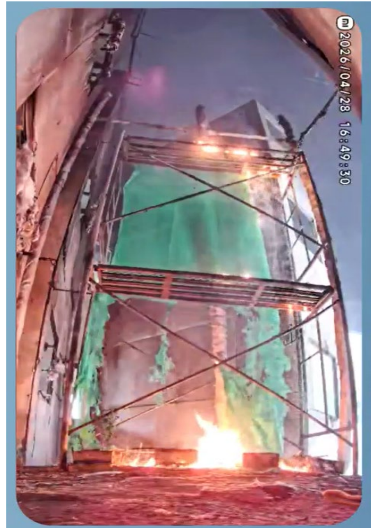
Photo 2-10 (z): Fire Spread on Sample 4 (Wang Chi) (26 min)
