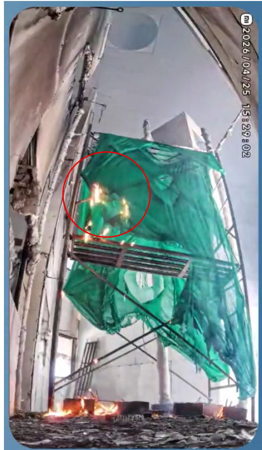
Photo 2-9 (b): Extensive Fire Spread on Sample 4 (Wang Chi)
