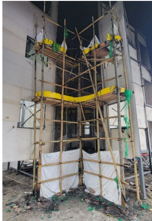
Photo 2-18 (d): Post-Fire Condition in Test 12 using Safety Nets collected Wang Chi House and FR Canvas
