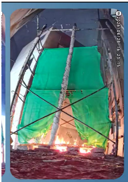
Photo 2-10 (a): Fire Spread on Sample 3 (Non-FR) (2 min)
