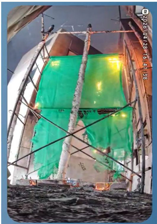
Photo 2-10 (s): Fire Spread on Sample 3 (Non-FR) (20 min)
