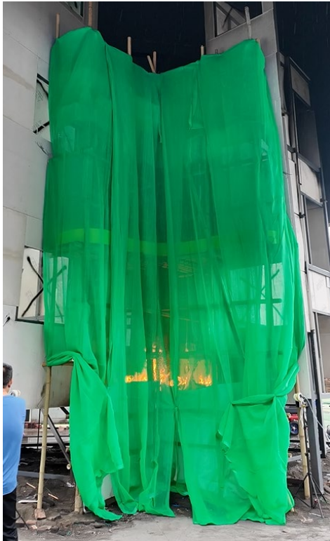
Photo 2-18 (a): No Fire Spread along Safety Nets in Test 11
