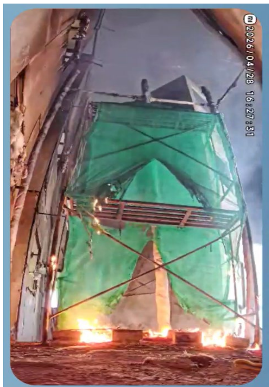
Photo 2-10 (f): Fire Spread on Sample 4 (Wang Chi) (6 min)
