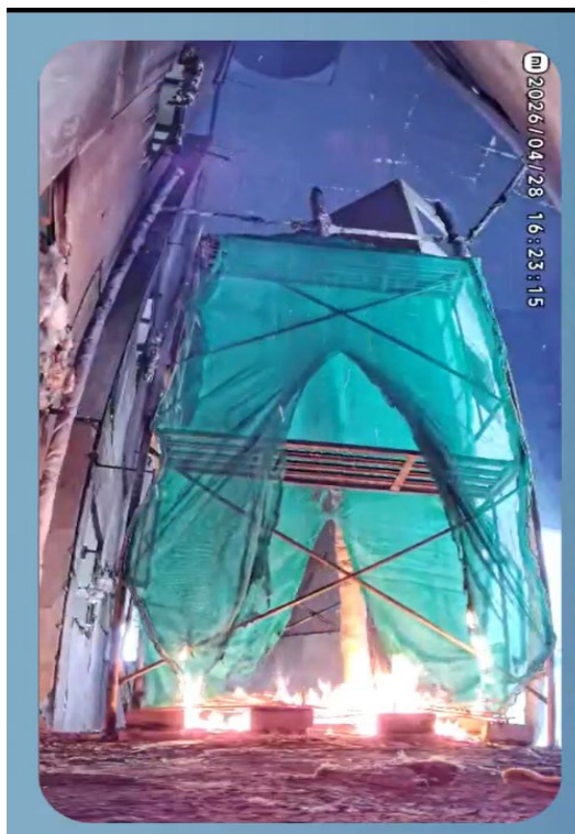
Photo 2-10 (b): Fire Spread on Sample 4 (Wang Chi) (2 min)
