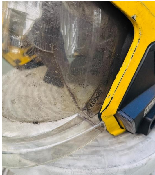
Photo 9-16 (b): Crack on Visor
