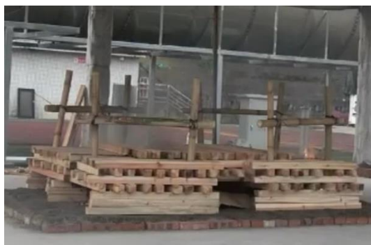
Photo 7-2 (a): Setup of Wooden Cribs as the Fire Source
