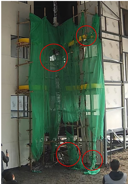
Photo 2-16 (c): Secondary Ignition in Test 3 [Sample 1 (Uncertified)]
