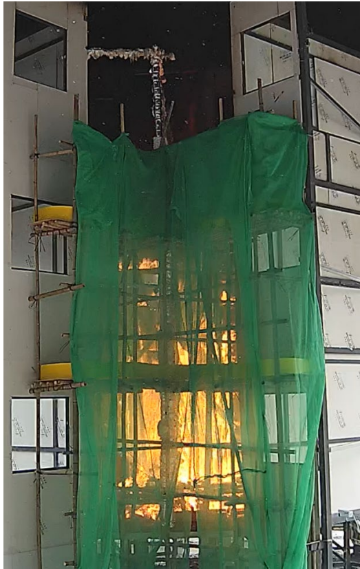
Photo 2-2 (a): Fully Developed Fire in Test 3 (Uncertified Safety Nets)
