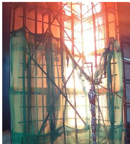
Photo 7-3 (b): The Fire Condition at 34 Mins With HRR Peaked at 29 MW
