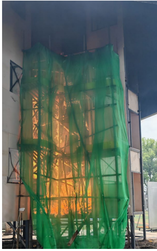
Photo 2-12 (b): Full Developed Fire in Test 8 using non-FR Safety Nets
