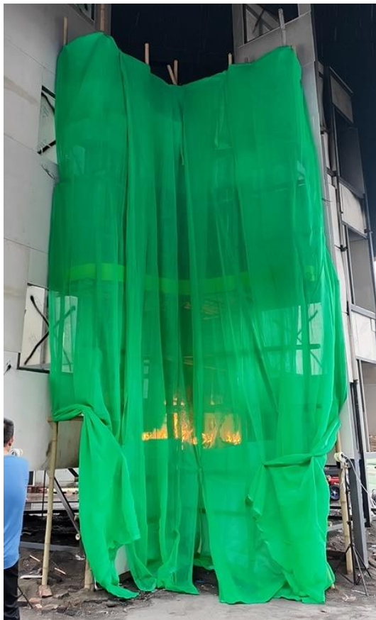
Photo 7-6 (a): No Fire Spread Along Safety Nets in Test 11
