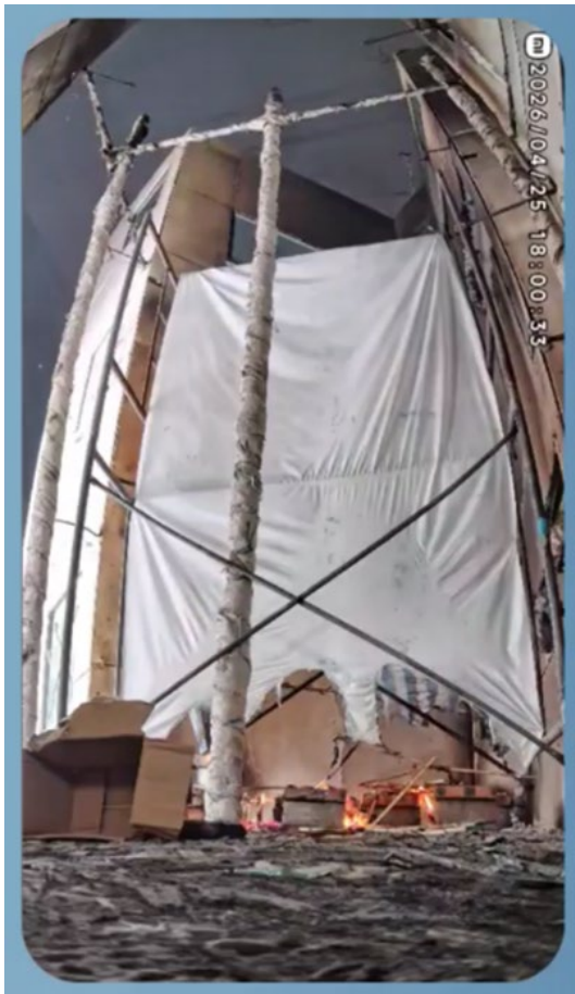
Photo 2-10 (ac): Limited Fire Damage on FR Canvas (White Color)
