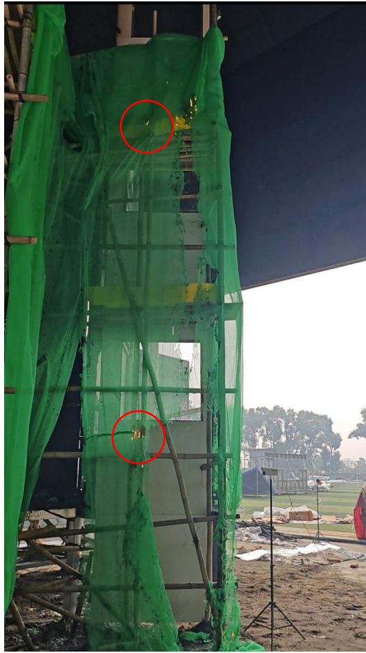
Photo 2-17 (b): Flaming Droplets Dripping and Spreading Fire
