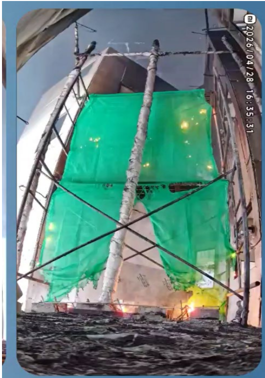
Photo 2-10 (m): Fire Spread on Sample 3 (Non-FR) (14 min)
