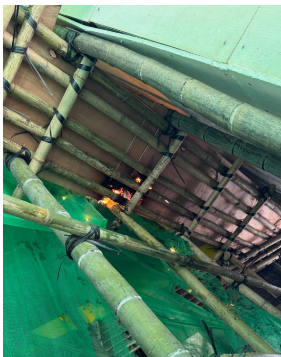
Photo 2-11 (a): Fire Spread in Test 1 Using Uncertified Safety Nets
