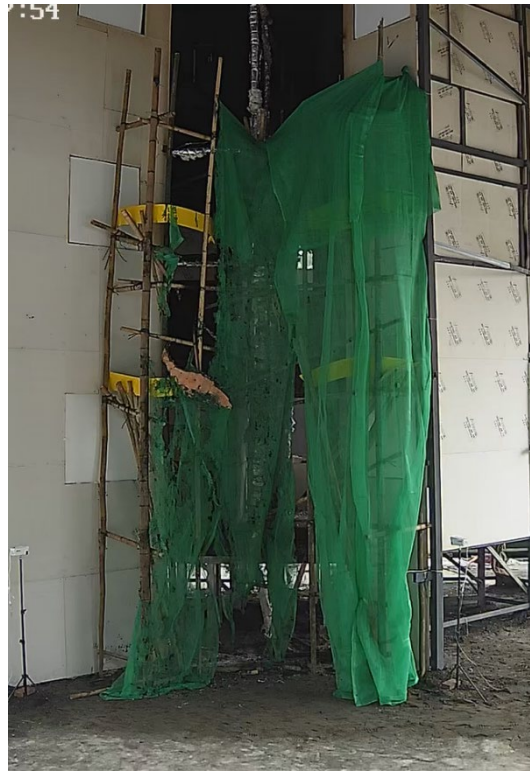
Photo 2-16 (f): Post-Fire Condition in Test 5 [Sample 1 (Uncertified)]
