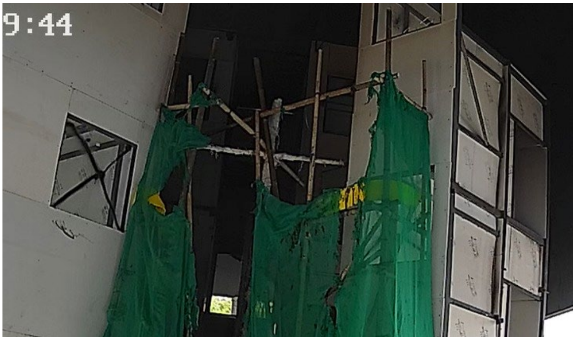
Photo 2-12 (g): Seriously Damaged Safety Nets in Test 8
