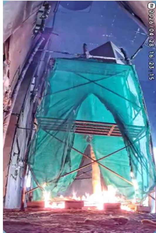
Photo 7-4 (g): Fire Spread on Sample 4 (Wang Chi) (2 mins)
