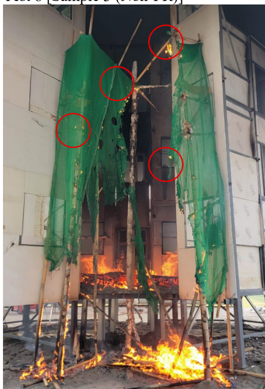
Photo 2-16 (k): Secondary Ignition in Test 9 [Sample 4 (Wang Chi House)]
