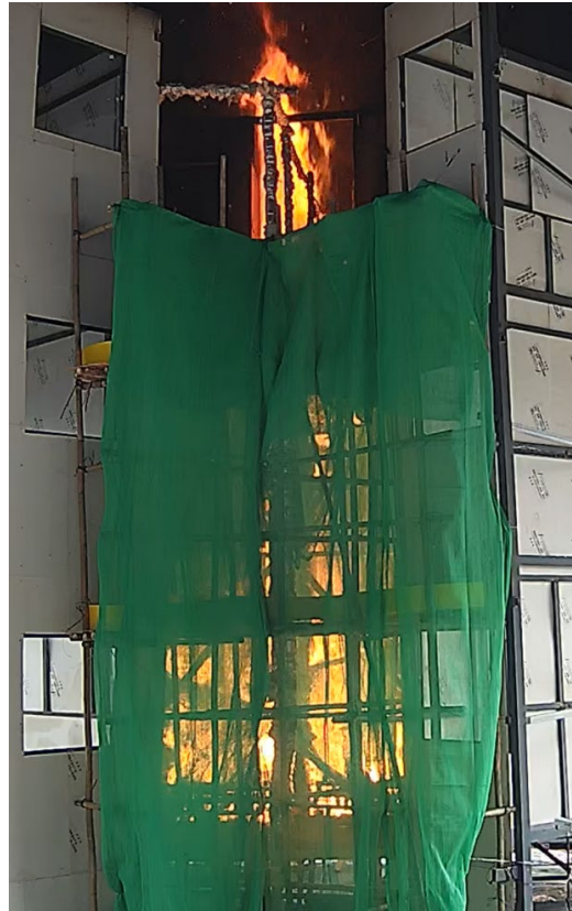
Photo 2-2 (b): Fully Developed Fire in Test 4 (FR Safety Nets)
