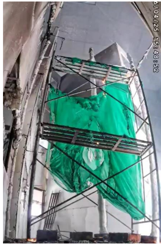
Photo 7-4 (e): Post-Fire Condition of Sample 4 (Fully Consumed)
