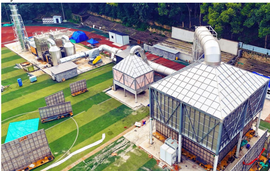
Fig. 2.4 20MW and 5MW cone calorimeter
