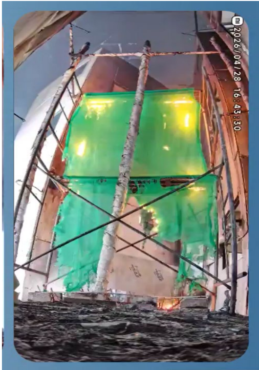
Photo 2-10 (u): Fire Spread on Sample 3 (Non-FR) (22 min)
