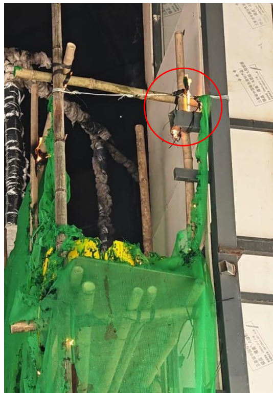
Photos 7-5 (c) & (d): Flaming Droplets Igniting Nylon Strips
