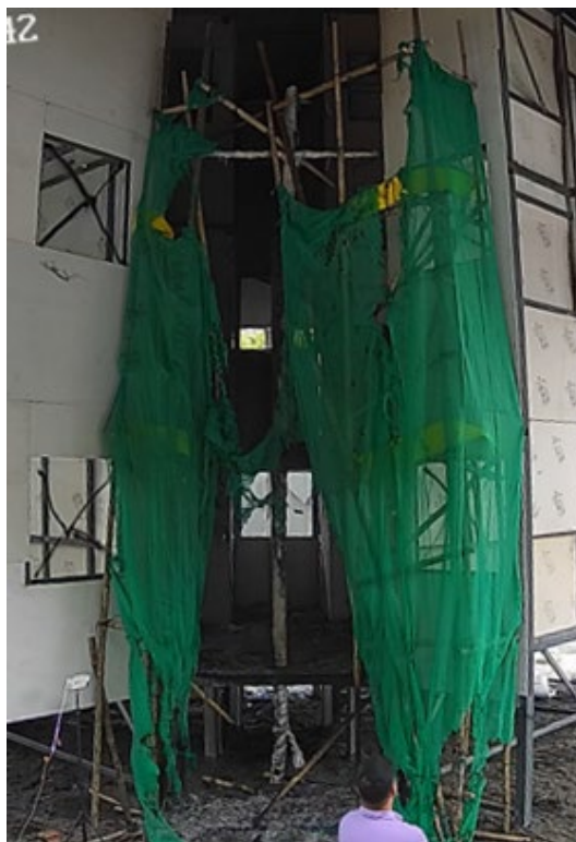
Photo 2-16 (j): Post-Fire Condition in Test 8 [Sample 3 (Non-FR)]
