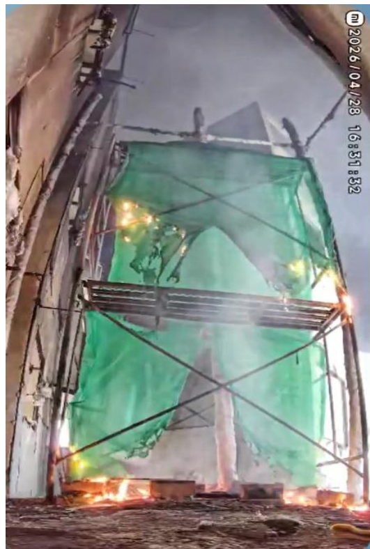
Photo 7-4 (i): Fire Spread on Sample 4 (10 mins)
