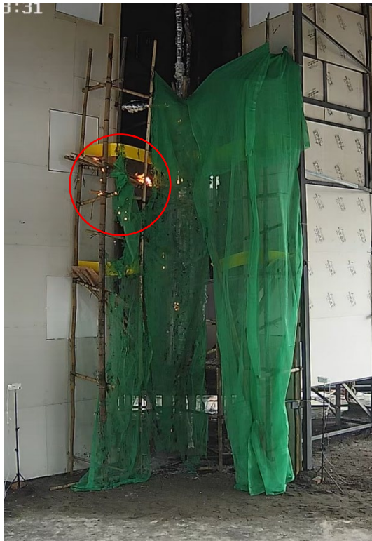
Photo 2-16 (e): Secondary Ignition in Test 5 [Sample 1 (Uncertified)] 34
