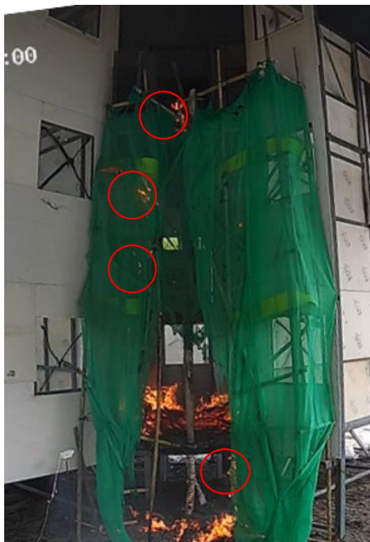
Photo 2-16 (i): Secondary Ignition in Test 8 [Sample 3 (Non-FR)]
