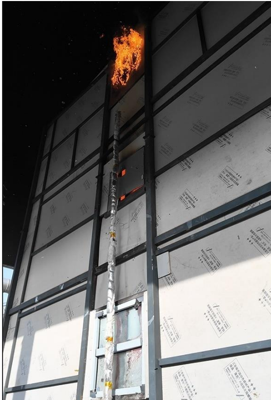
Photo 10-8 (b): Ignition of Wooden Board (4 Mins 40 Secs)
