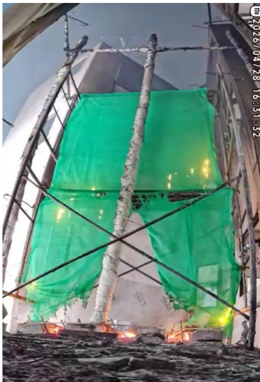
Photo 7-4 (h): Fire Spread on Sample 3 (10 mins)
