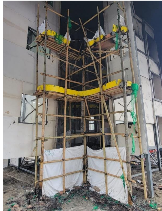
Photo 7-6 (d): Post-Fire Condition in Test 12 Using Safety Nets Collected From Wang Chi House and FR Canvas
