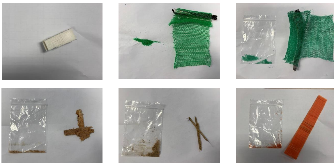
Fig. 1.2 Image of sample preparation process for TGA which involve grinding the material to powder form.
