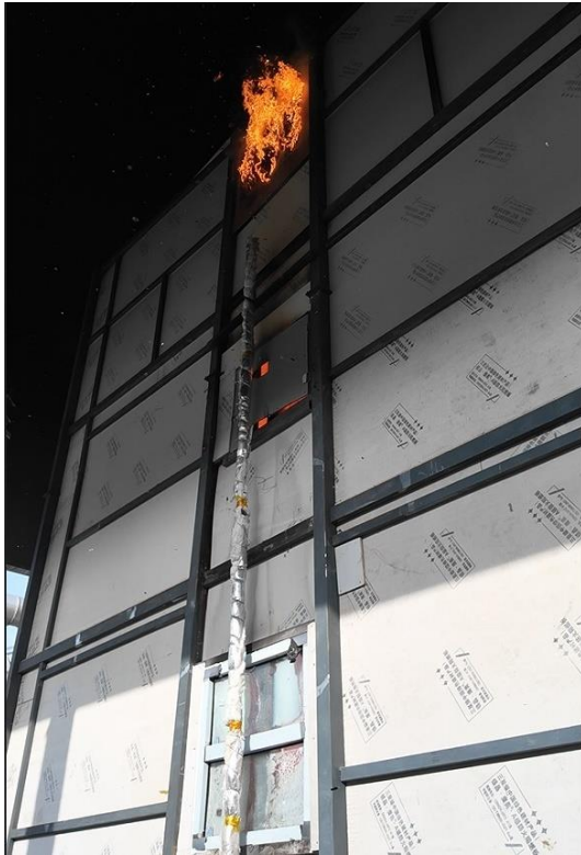
Photo 7-8 (a): Ignition of Wooden Board (4 Mins 40 Secs)
