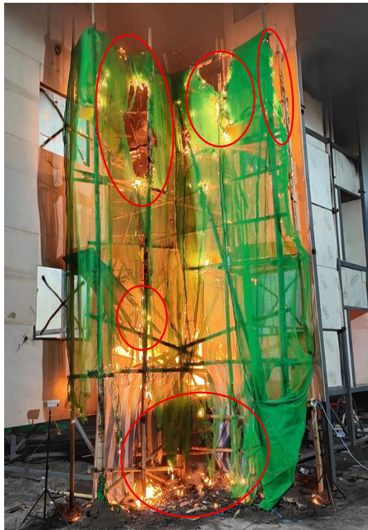
Photos 7-6 (e) & (f): Fire Spread Along Safety Nets in Test 13
