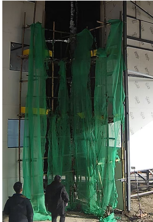
Photo 2-16 (b): Post-Fire Condition in Test 1 [Sample 1 (Uncertified)]
