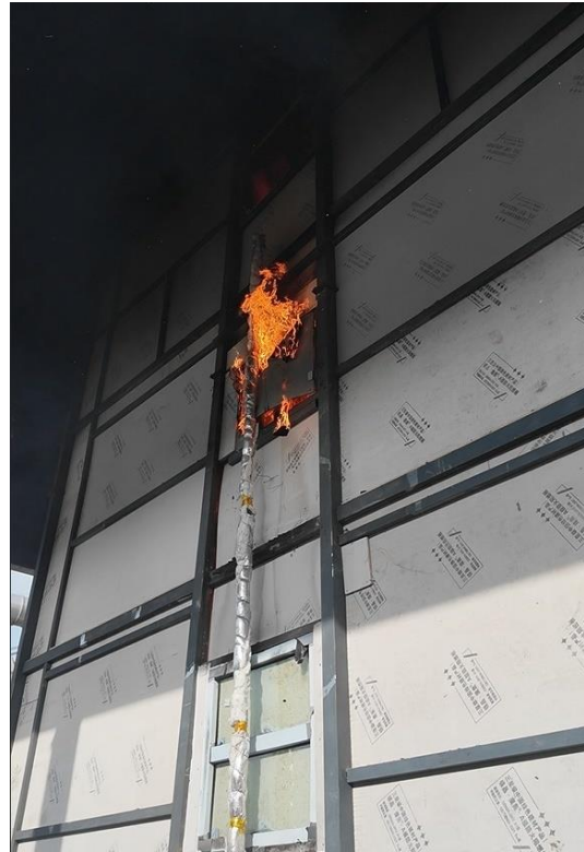
Photo 10-8 (c): Ignition of Aluminium Composite Panel (7 Mins 49 Secs)
