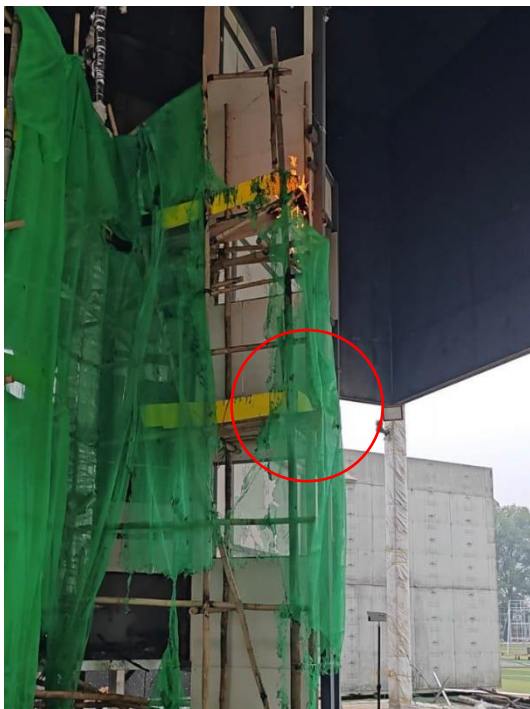
Photos 7-5 (g) & (h): Flaming Droplets Causing Further Fire Propagation
