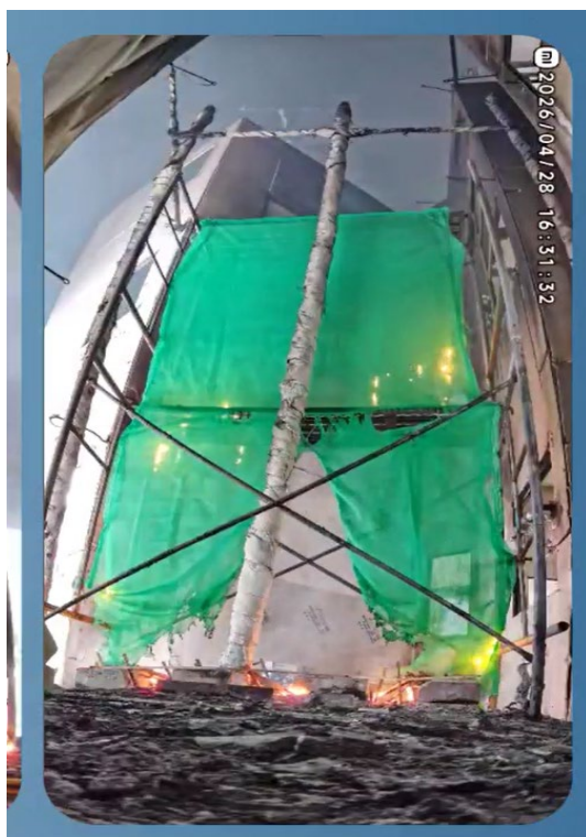
Photo 2-10 (i): Fire Spread on Sample 3 (Non-FR) (10 min)
