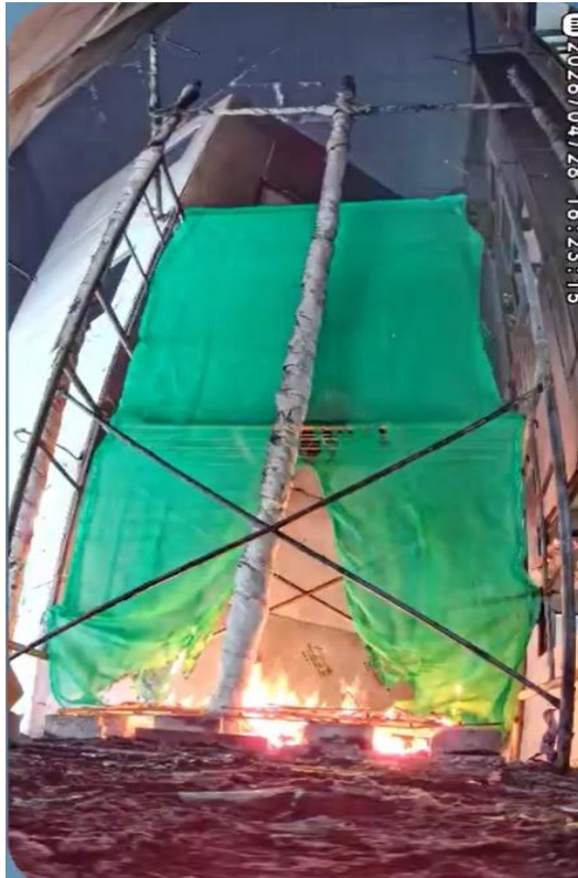
Photo 7-4 (f): Fire Spread on Sample 3 (Non-FR) (2 mins)
