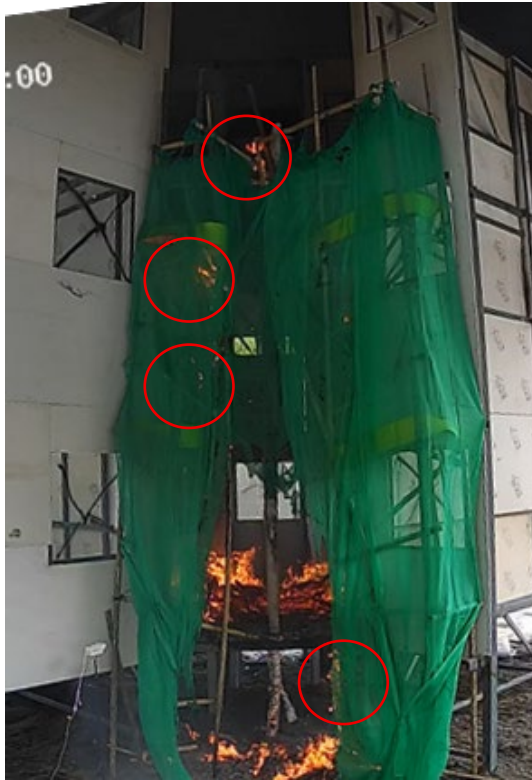
Photo 2-12 (e): Secondary Ignition Occurred in Test 8
