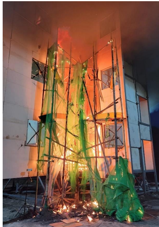
Photos 7-6 (e) & (f): Fire Spread Along Safety Nets in Test 13
