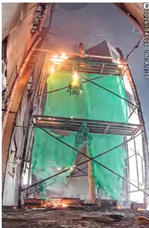
Photo 7-4 (k): Fire Spread on Sample 4 (20 mins) 92
