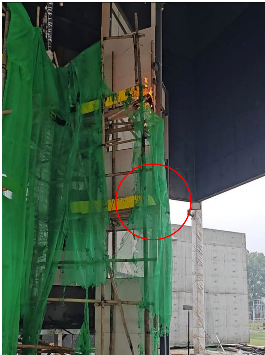
Photos 2-17 (g) & (h): Flaming Droplets Causing Further Fire Propagation.
