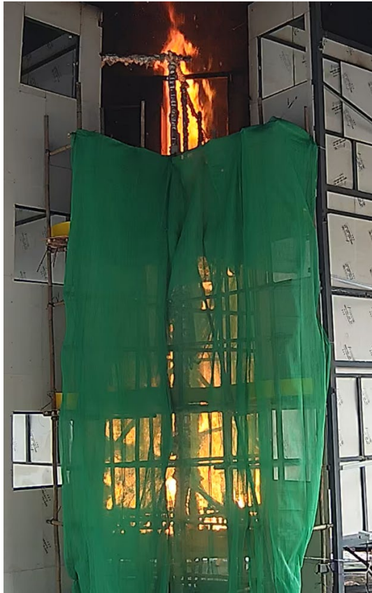
Photo 2-12 (a): Full Developed Fire in Test 4 using FR Safety Nets
