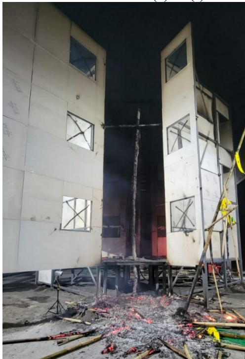
Photo 2-18 (g): Post-Fire Condition in Test 13 using Safety Nets collected Wang Chi House and non-FR Canvas
