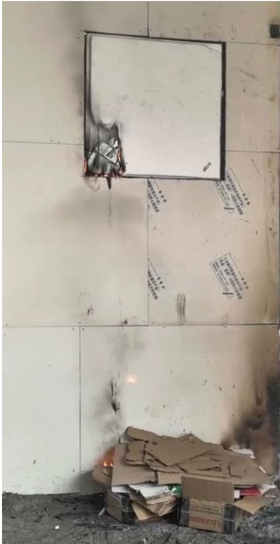
Photo 2-13 (a): Formation of Burning Droplets from the Ignited Polystyrene Window Covers
