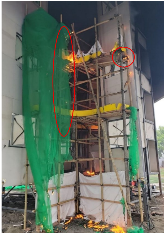
Photo 2-18 (c): Fire Spread along Safety Nets in Test 12
