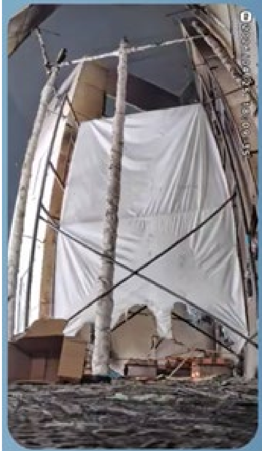
Photo 2-10 (ae): Post-Fire Condition of FR Canvas (Partially Intact)
