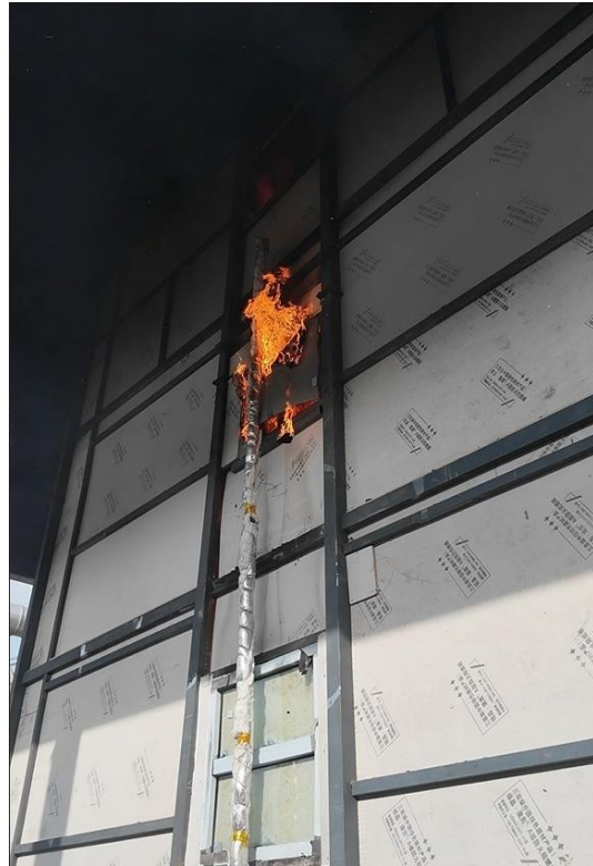
Photo 7-8 (b): Ignition of Aluminium Composite Panel (7 Mins 49 Secs)
