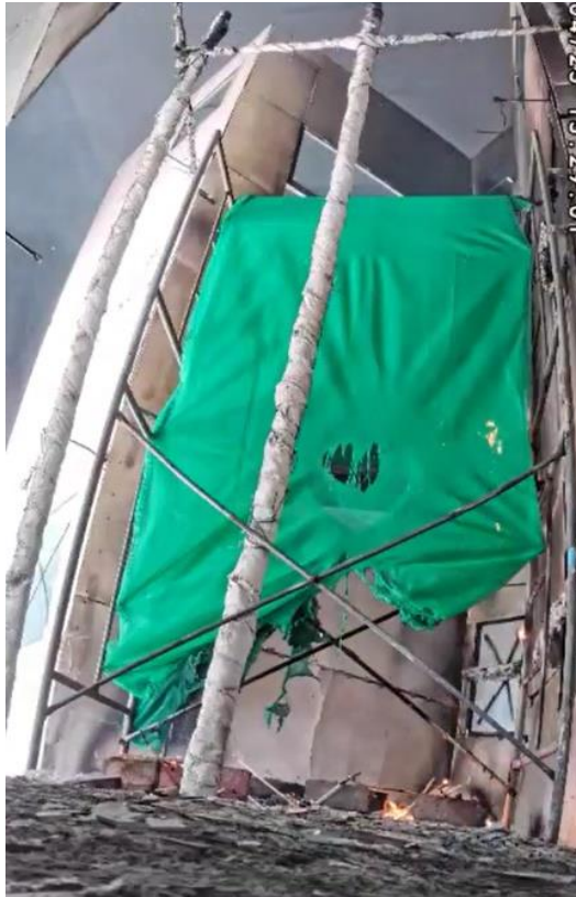
Photo 7-4 (b): Limited Fire Damage on Sample 2 (FR)
